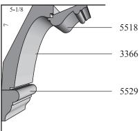
**Fig. 33**Crown Buildup to emphasize ceiling height
